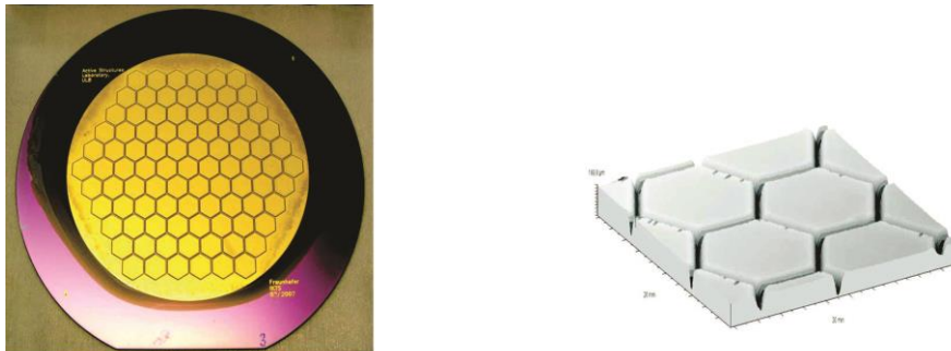
Fig. 5 Deformable mirror made of a 150 mm Silicon wafer covered on its back side with an array of screen printed PZT actuators with honeycomb electrodes acting in the d_{31} mode
